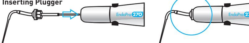
Note: The mouth of the Heating Unit has 6 different slots for inserting the Plugger. Select the appropriate one based on your preferred orientation of the Heater Switches in relation to the Plugger tip.
